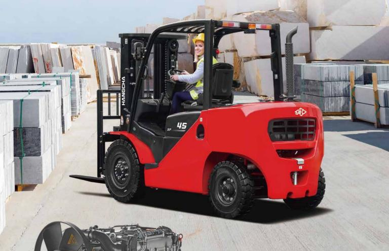
With Hangcha you can meet all Stage V/Tier 4f emissions standards which provides customer demands for value, innovation and performance. The technologies include common rail fuel systems, diesel oxidation catalysts (DOC) and diesel particulate filters (DPF). Designed and optimised to every engine model, our forklift truck maximises efficiency and reliability.
